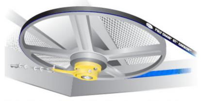
Gates Draftguard prevents fan drives from rotating in the reverse direction. At the core of our product is a high-torque, one-way clutch. The flange plate is engineered to mount to either Taper-Lock® or QD® bushings used in ACHE belt drive systems. The torque arm enables mounting to the frame for complete protection. Draftguard anti-rotation device is flat, allowing it to fit within most fan guards.
